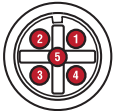
Male, 5-pin (DeviceNet micro connector) pin-out as viewed from the end of the sensor
